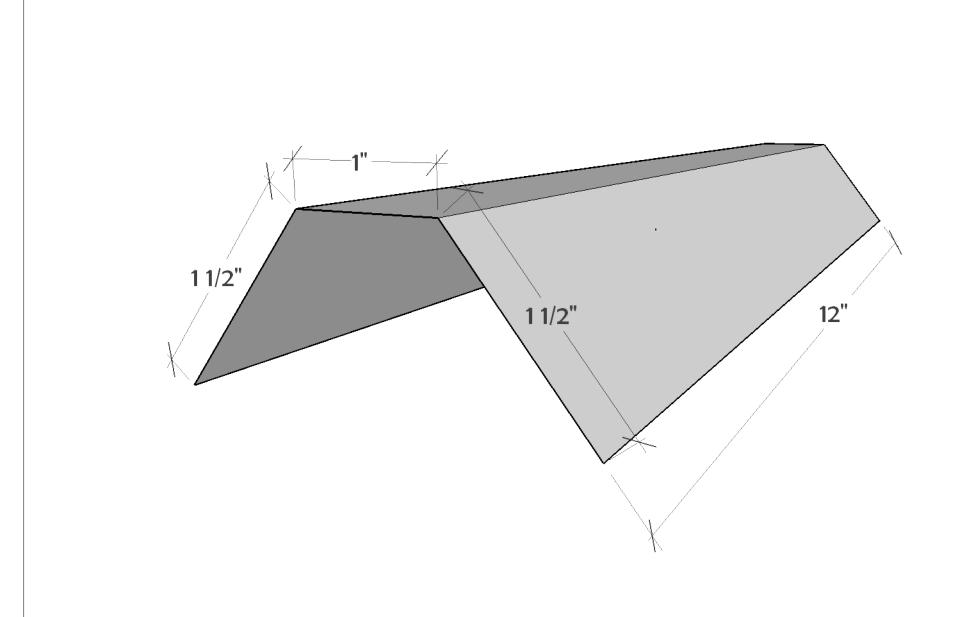
Part No: 38 Gutter Support (PBR) Stretch: 4"
