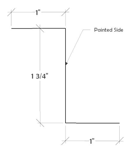
Part No: 83 Lokseam Z-Bar Closure Stretch: 3 3/4"
