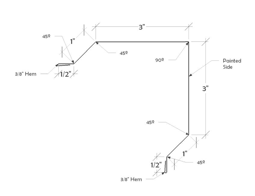
Part No: 48 3 x 3 Corner Rake (XRib) Stretch: 9 3/4"
