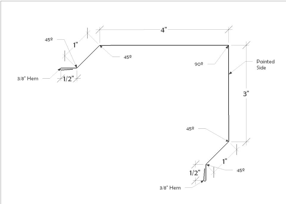
Part No: 43 3 x 4 Corner Rake (XRib) Stretch: 10 3/4"
