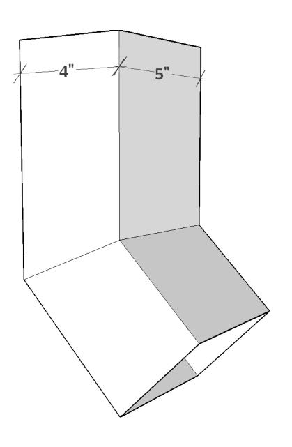
Part No: 41 4" x 5" Downspout Elbow (45° or 90°) Stretch: 6 3/4"
