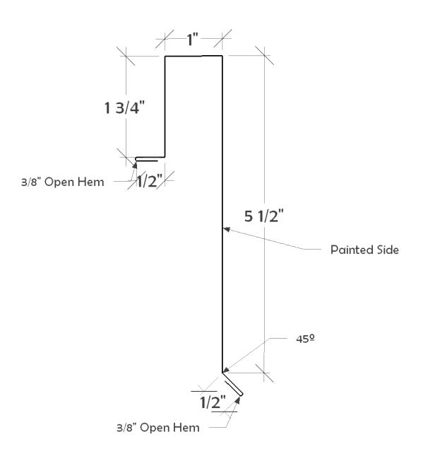
Part No: 81 Lokseam Rake Trim Stretch: 10"
